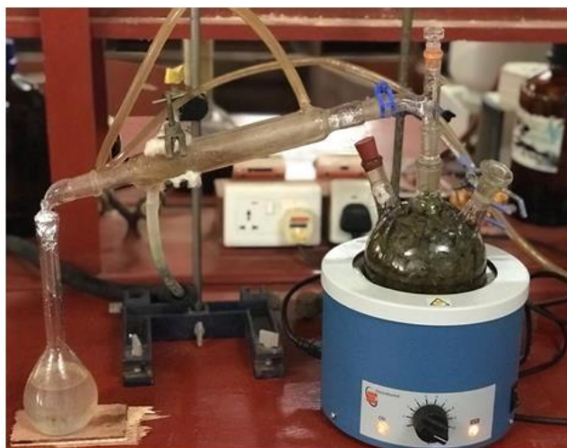
Figure 1 A Hydro-Distillation Setup
